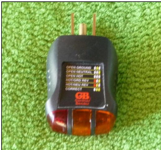
Figure 5-4 Simple Circuit Outlet Polarity Tester
