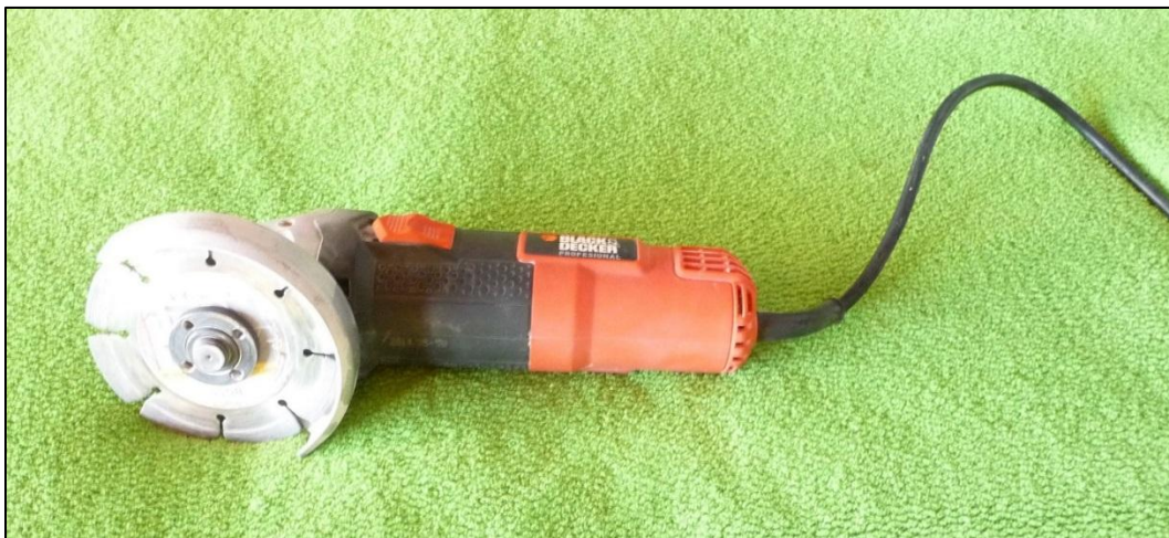
Figure 5-7 Cutter with Diamond Blade
