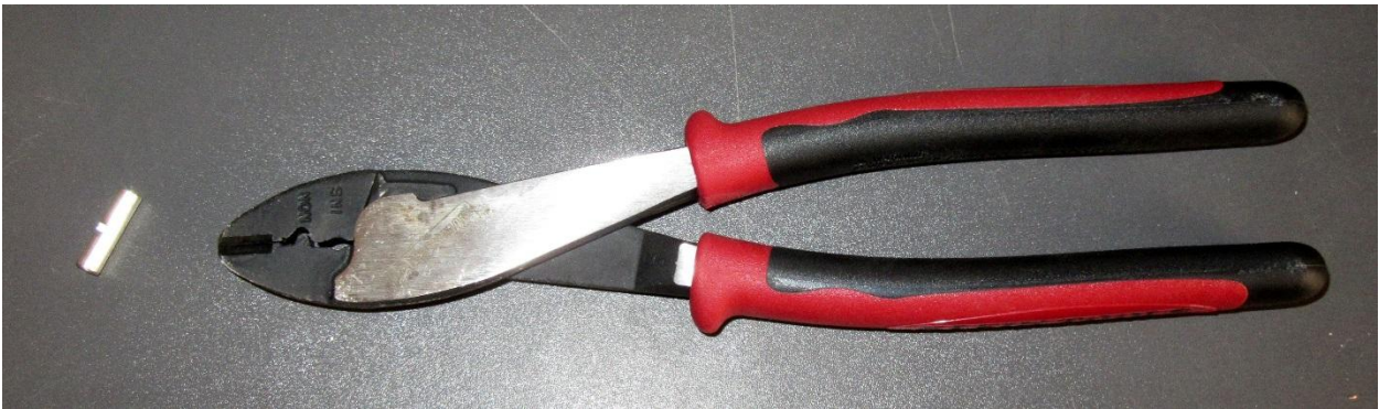
Figure 5-9 AWG10 to 12 Crimp and Crimper
