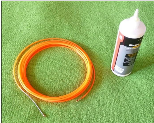
Figure 5-6 Wire puller and Lubricant
