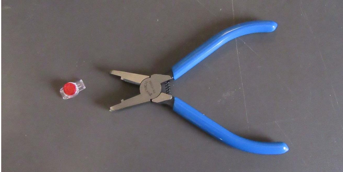
Figure 5-10 AWG 19 to 26 Splice and Crimp Tool
