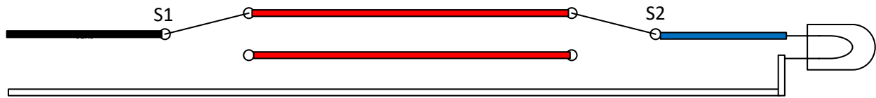
Figure 2-19 US Method for Wiring Three-Way Light Circuit
