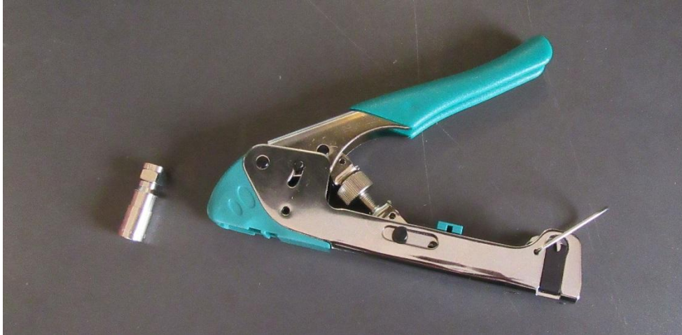
Figure 5-12 RG6 Coax Connector and Crimp Tool
