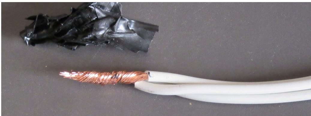
Figure 2-10 Twisted Connection without Tape
