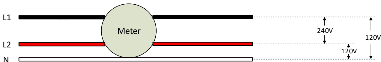
Figure 2-1 Two Phase Line Voltages
