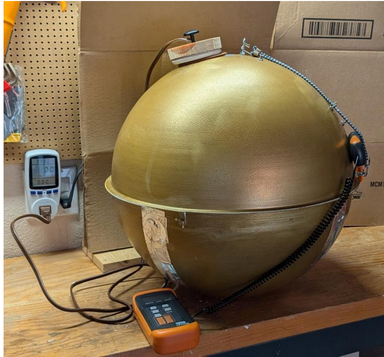
Ulbricht Sphere in Operation
