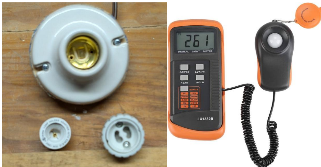
E26 Socket with Adapters (left), Remote Readout Light Meter (right)
