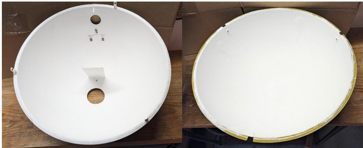
Inside of Ulbricht Sphere
